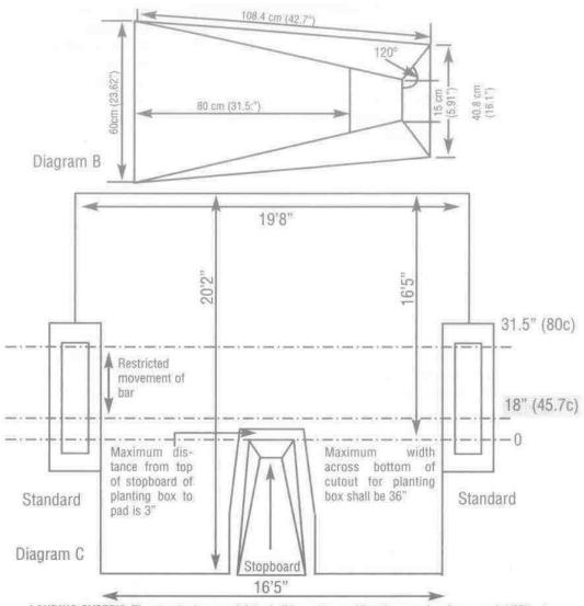
**LANDING SYSTEM**: The standards or uprights shall be set to position the crossbar from a point 18 inches (45.7c) beyond the vertical plane of the top of the stopboard, up to a maximum distance of 31.5 inches (80c) in the direction of the landing surface.
